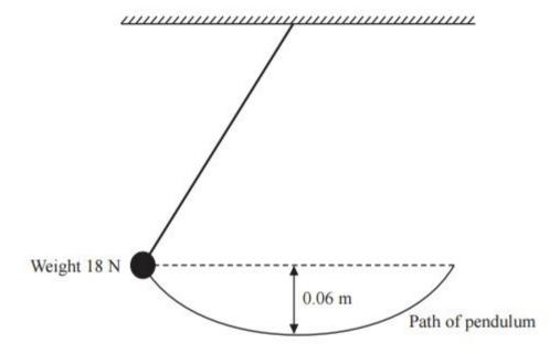
A pendulum consists of an 18 N weight attached to a piece of string. The weight is released from the position shown in the diagram. The speed in m s<sup>-1</sup> at the bottom of the swing is given by
