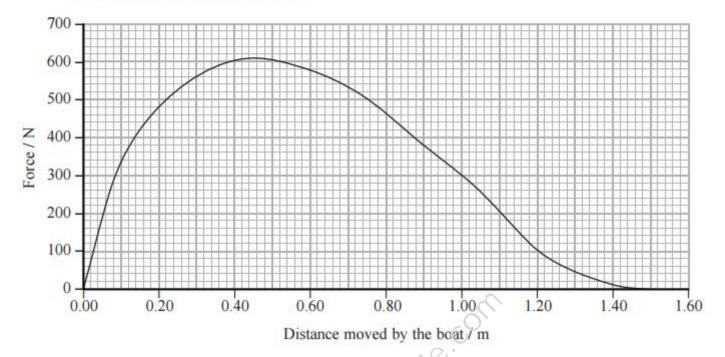
(i) Use the graph to show that the work done on the boat during one stroke is about 500 J.
