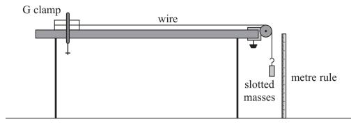
Masses were added up to a maximum of 3.30 kg. Each time a mass was added the extension of the wire was calculated.
