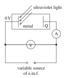
When ultraviolet light of a particular frequency is shone on the metal a current is produced. Current is produced for all values of potential difference when Q is positive. If Q is negative there is a p.d. beyond which there is no current. The magnitude of this p.d. is called the stopping potential  $V_{\rm s}$ .
