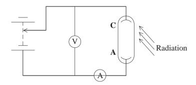
(a) A light is shone onto the cathode C and a potential difference is applied between the cathode and the anode A of the photocell. A sensitive ammeter is used to detect any current that flows.
