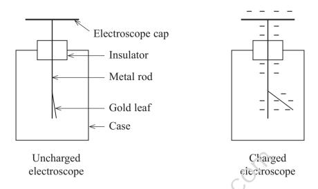
A gold leaf electroscope can be used to demonstrate the photoelectric effect. A clean zinc plate is placed onto the cap of the electroscope and the plate and electroscope are charged negatively. Ultraviolet radiation is shore onto the zinc plate.
