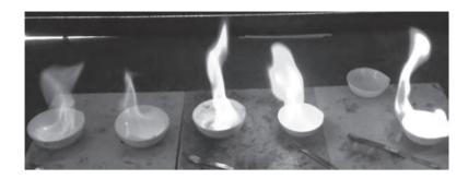
Flame tests are used to identify the elements present in some chemical compounds. The compounds produce different coloured flames when vaporised. This is because different elements produce spectra containing light with different wavelengths.
