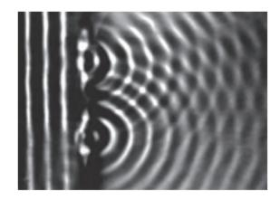
Plane waves travelling from the left strike a barrier with two gaps.
