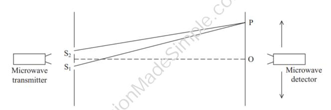
The detector is moved from O in the direction of the upwards arrow. The first position where the signal is a minimum is P.
