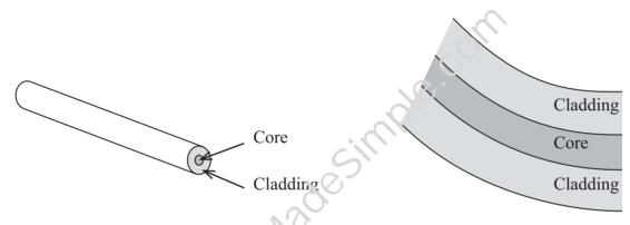
speed of light in the core =  $1.96 \times 10^8$  m s<sup>-1</sup> speed of light in the cladding =  $2.03 \times 10^8$  m s<sup>-1</sup>
