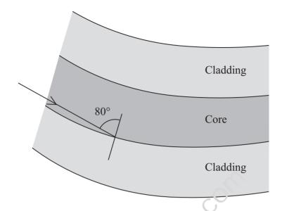
State what happens to this ray of light when it is incident on the core-cladding boundary as shown.
