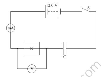
The capacitor is initially uncharged and the switch is closed at time t=0. The graph shows how the potential difference  $V_{\rm R}$  across the resistor varies with time t.
