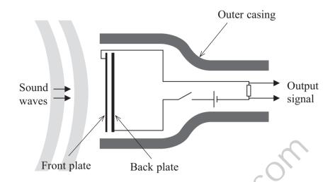
The sound waves cause the flexible front plate to vibrate and change the capacitance. Moving the plates closer together increases the capacitance. Moving the plates further apart decreases the capacitance.
