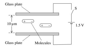
The molecules are positive at one end and negative at the other. They are normally aligned parallel with the glass plates as shown.
