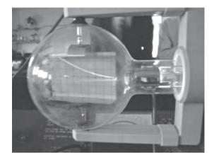
A potential difference (p.d.) of 4800 V is applied between the cathode and anode of the tube. The cathode is heated and electrons are emitted from its surface. These electrons are then accelerated from rest and pass through a hole in the anode.
