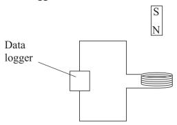
The data from the data logger is used to produce a graph of induced e.m.f. across the coil against time.
