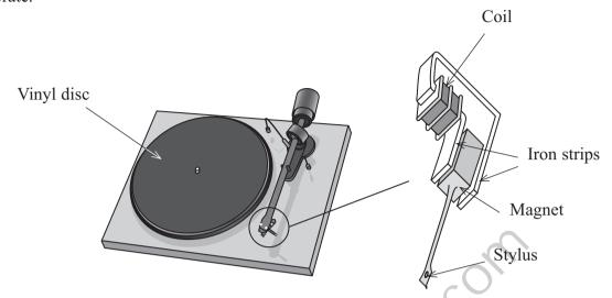
The stylus is attached to a small magnet which is near to a coil of wire. When the stylus vibrates, there is a potential difference across the terminals of the coil.
