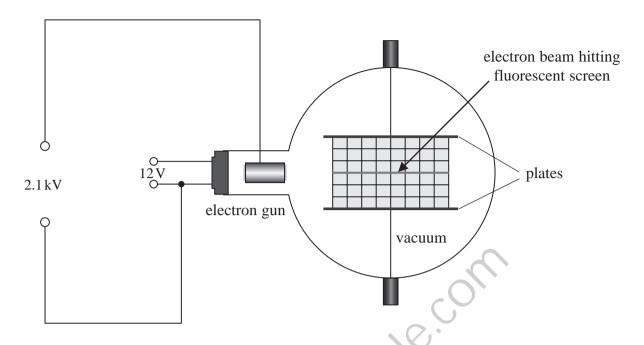
(a) The electron gun consists of a hot metal filament and a positively charged anode.
