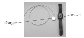
Induction charging does not require a metal connection between the charger and the device. The battery in the watch is charged by placing the watch on top of the charger.
