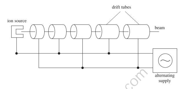
Explain how the linac produces a beam of high speed particles, making reference to the alternating supply and the lengths of the tubes.
