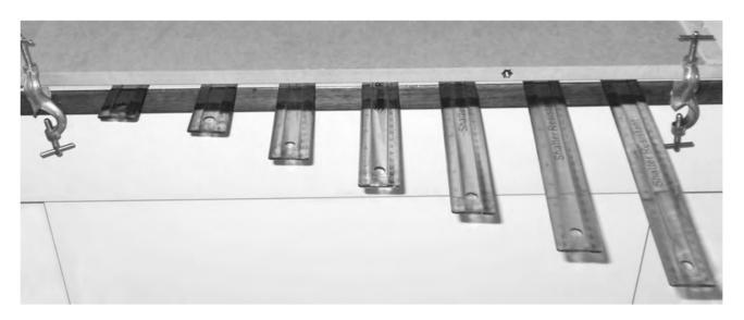
One end of each ruler is held flat on the desk whilst the other end is set into oscillation. Each ruler oscillates at a different frequency. Some of the rulers produce an audible sound.
