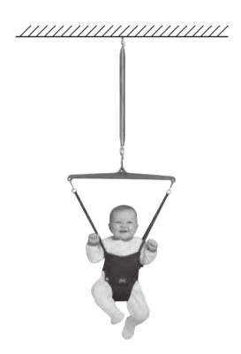
The height of the baby-bouncer is adjusted so that the baby's feet are a few centimetres above the floor when the baby is in equilibrium in the harness. If the baby is then displaced downwards and released, the system oscillates vertically with simple harmonic motion.
